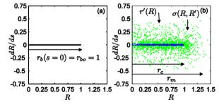
Figure 1: Beam phase-space structure in two distinct times of its dynamics inside the magnetic focusing channel. Panel (a) show beam phase-space at initial state s = 0 and (b) show beam phase-space after equilibrium is reached, at s = 796.3. Results have been obtained through numerical simulation with magnitude of inhomogeneity  $\eta = 0.5$  and with a matched envelope of  $r_b(s = 0) = r_{bo} = 1$ .
