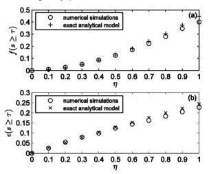
Figure 2: Comparison between results provided by numerical simulations and the exact analytical model as a function of magnitude of inhomogeneity  $\eta$ . Results are shown in (a) for the fraction *f* and in (b) for emittance  $\epsilon$ .
