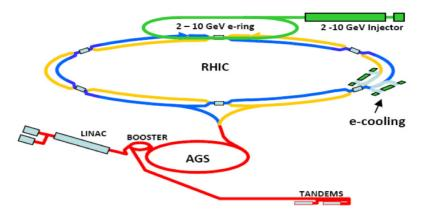
Figure 2: Schematic layout of the eRHIC ring-ring electron-ion collider [4].
