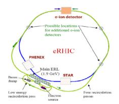
Figure 6: Schematic layout of the eRHIC linac-ring electron-ion collider [4].
