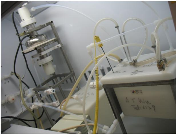
Figure 1: Vertical electropolishing system built for treating Nb SRF single cell cavities.
