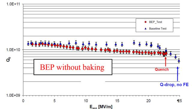
Figure 5: Excitation curves for a fine grain Nb single cell cavity treated by BEP using home-mixed acid.
