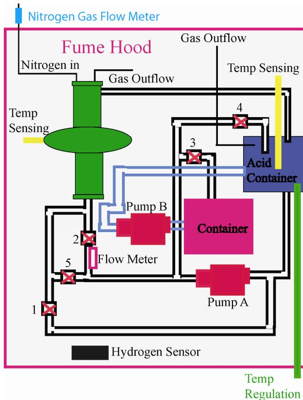
Figure 2: Schematic of the working principal of the vertical electropolishing system for Nb SRF single cell cavities (see text for more details).
