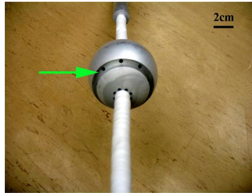
Figure 4: Ball shape cathode. The groove indicated by the arrow is designed to trap hydrogen generated during BEP.
