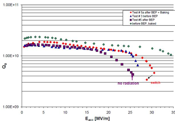
Figure 3: RF data of the first large grain Nb single cell cavity treated by the vertical EP system built at JLab.
