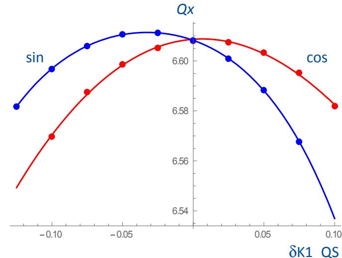
Tunes near half-integer vs. amplitude of sine and cosine modulation of QS and QL (13<sup>th</sup> harmonic). Calibration:
