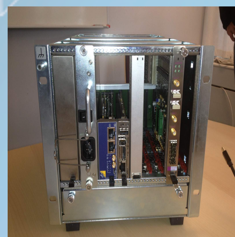
MTCA.4 electronics including Struck digitizer and NAT MCH
