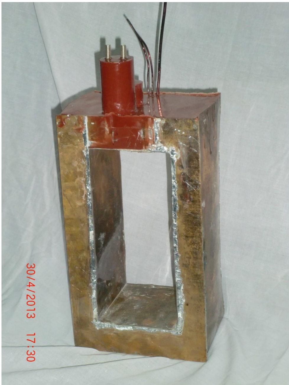
Construction of Epoxy Cast Secondary Winding
