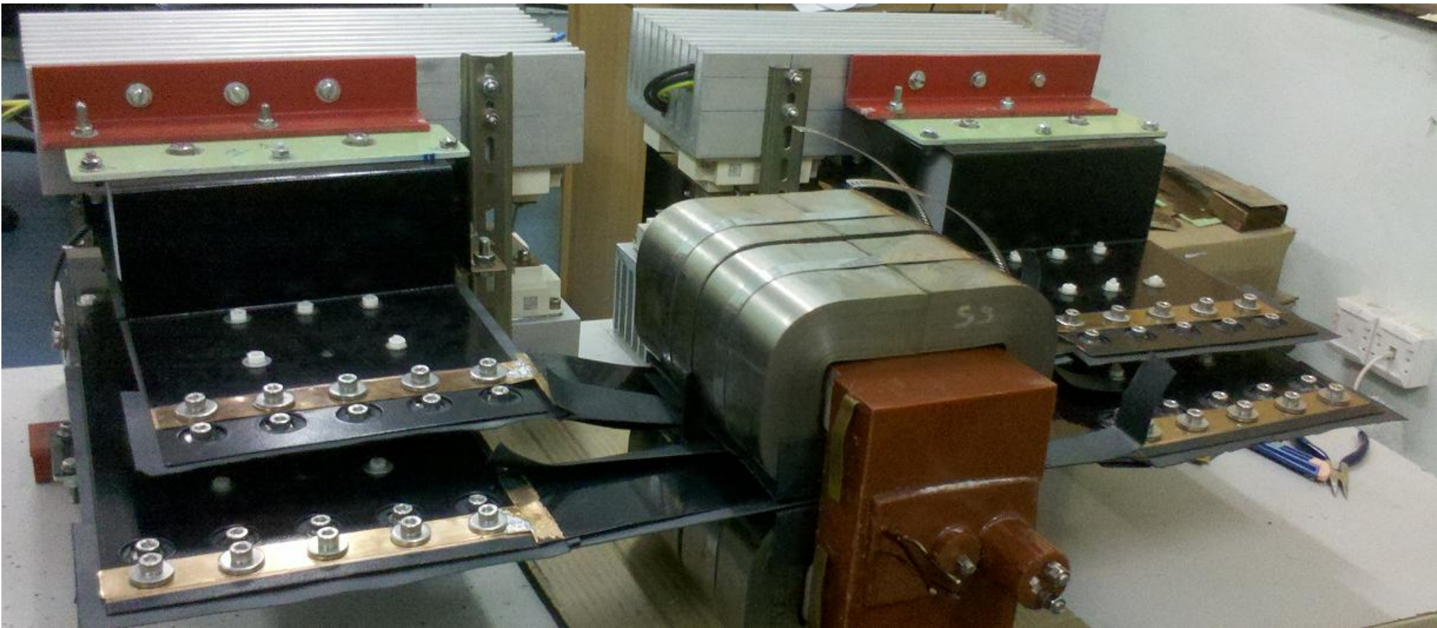
Different Views of the Discharging Circuit of the Prototype Modulator without the Load
