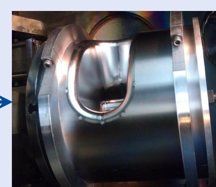
Tack weld while fixtured
