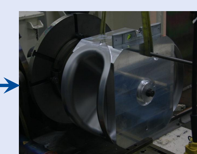
Tack weld while fixtured
