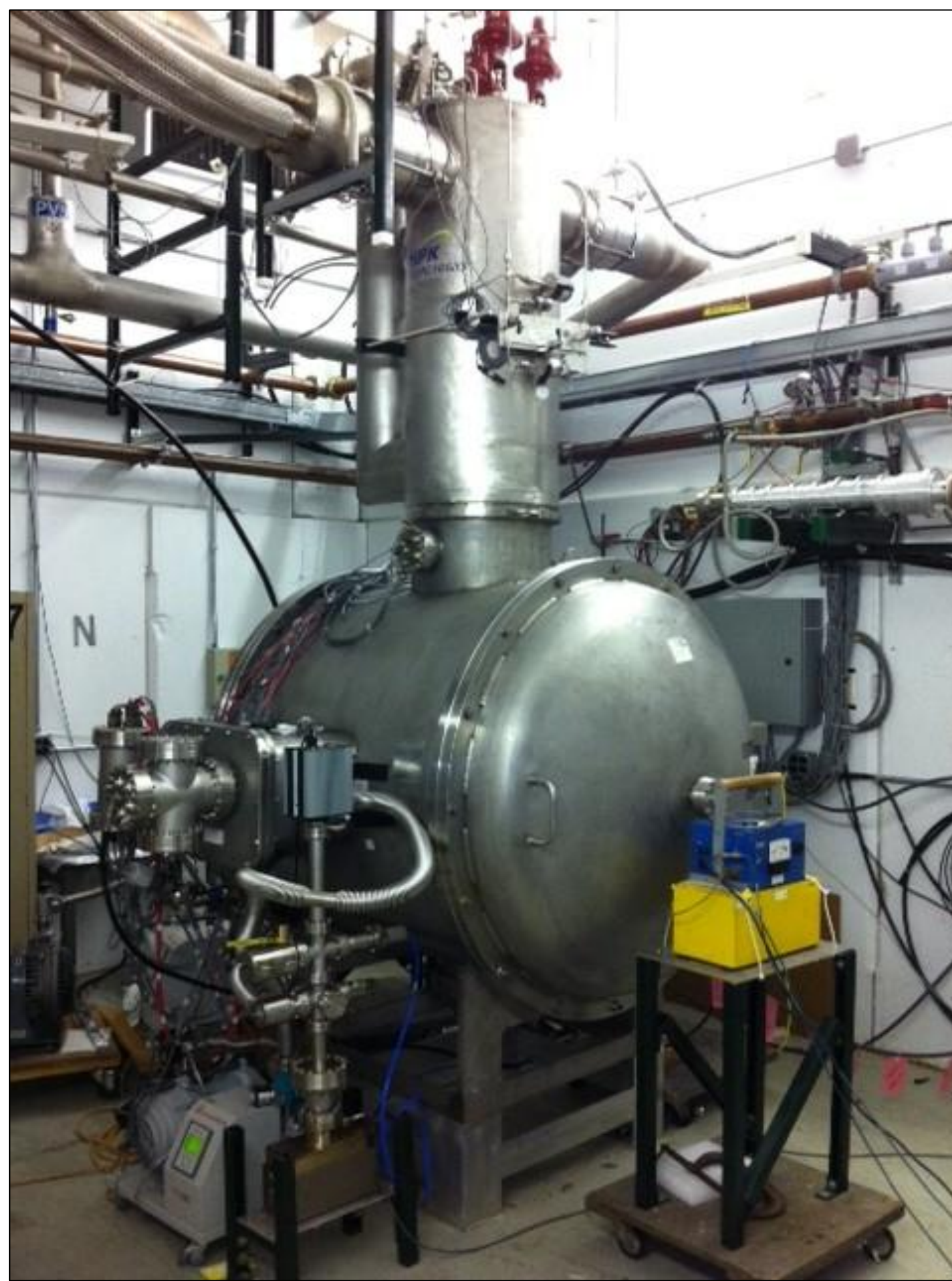
Spoke Test Cryostat with new 2 K feedcan
