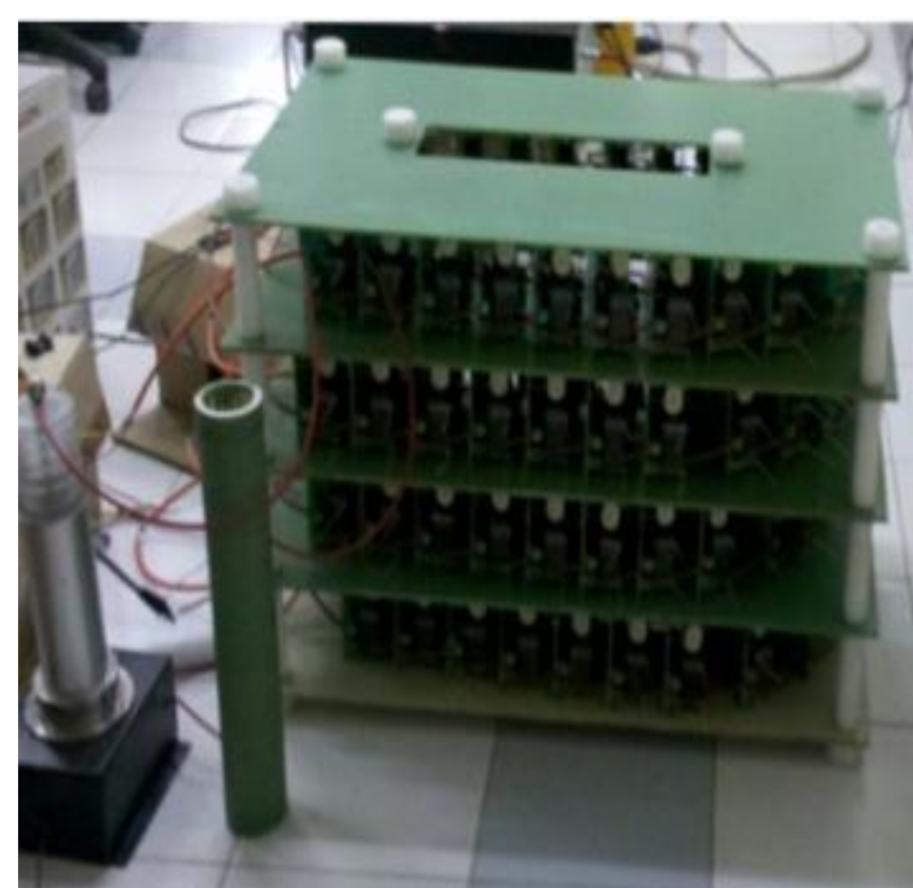
Marx adder (84-stage) and output of 40 kV on resistive load
