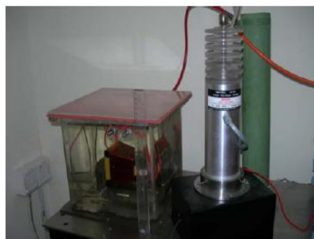
IGBT-based modulator with 90 kV output pulse
