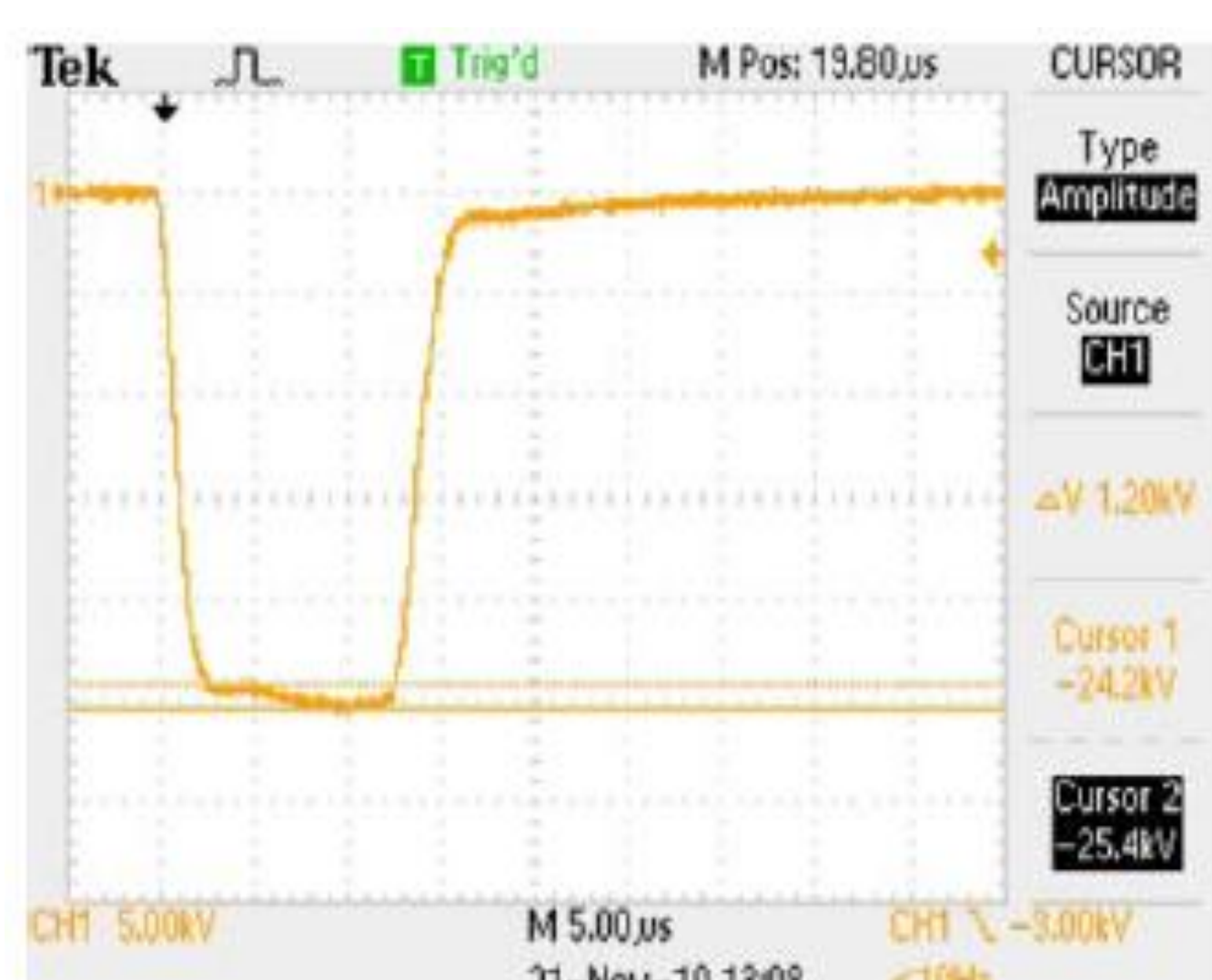
IGBT-based modulator with 90 kV output pulse
