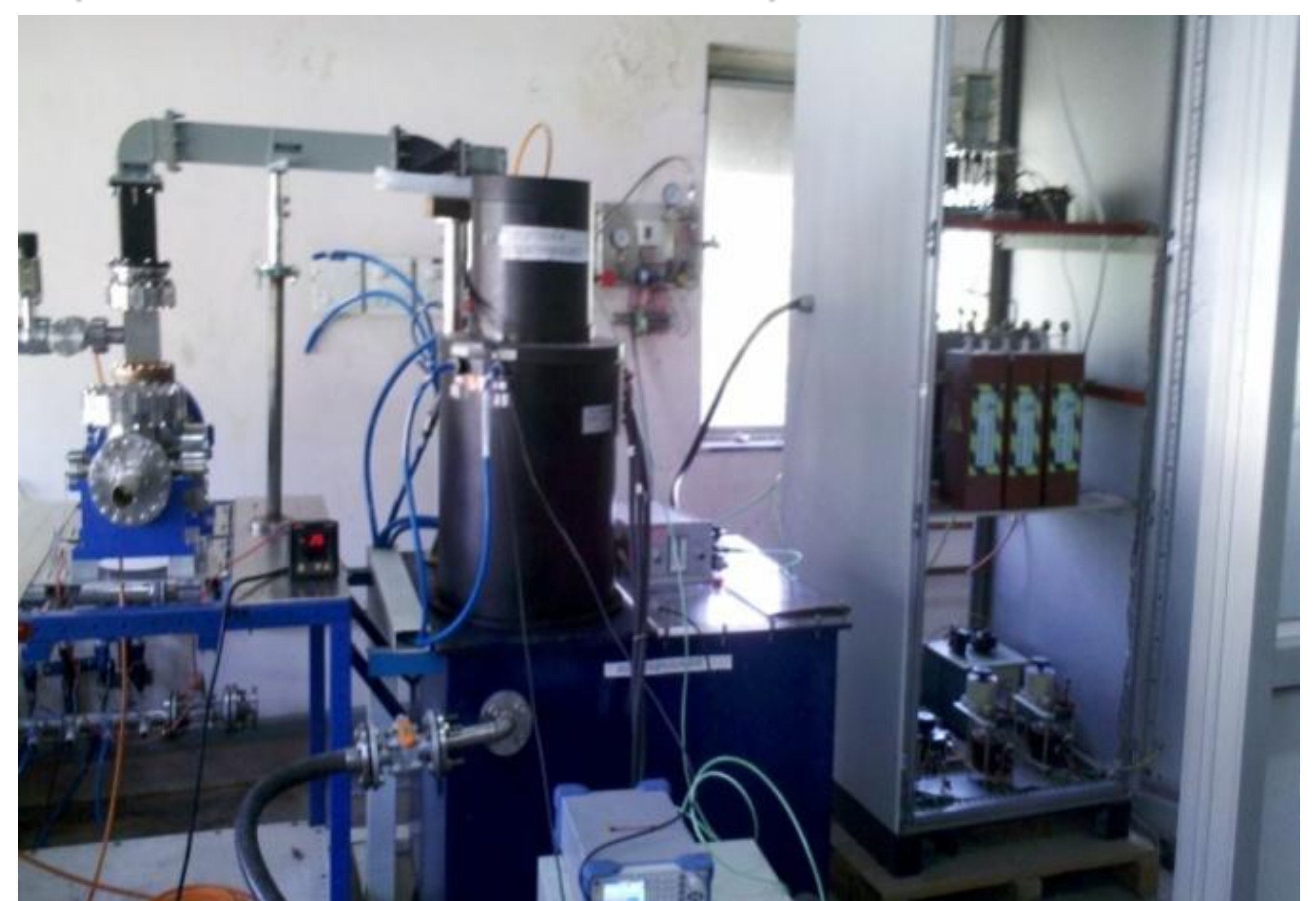
Modulator with single-beam klystron on test
