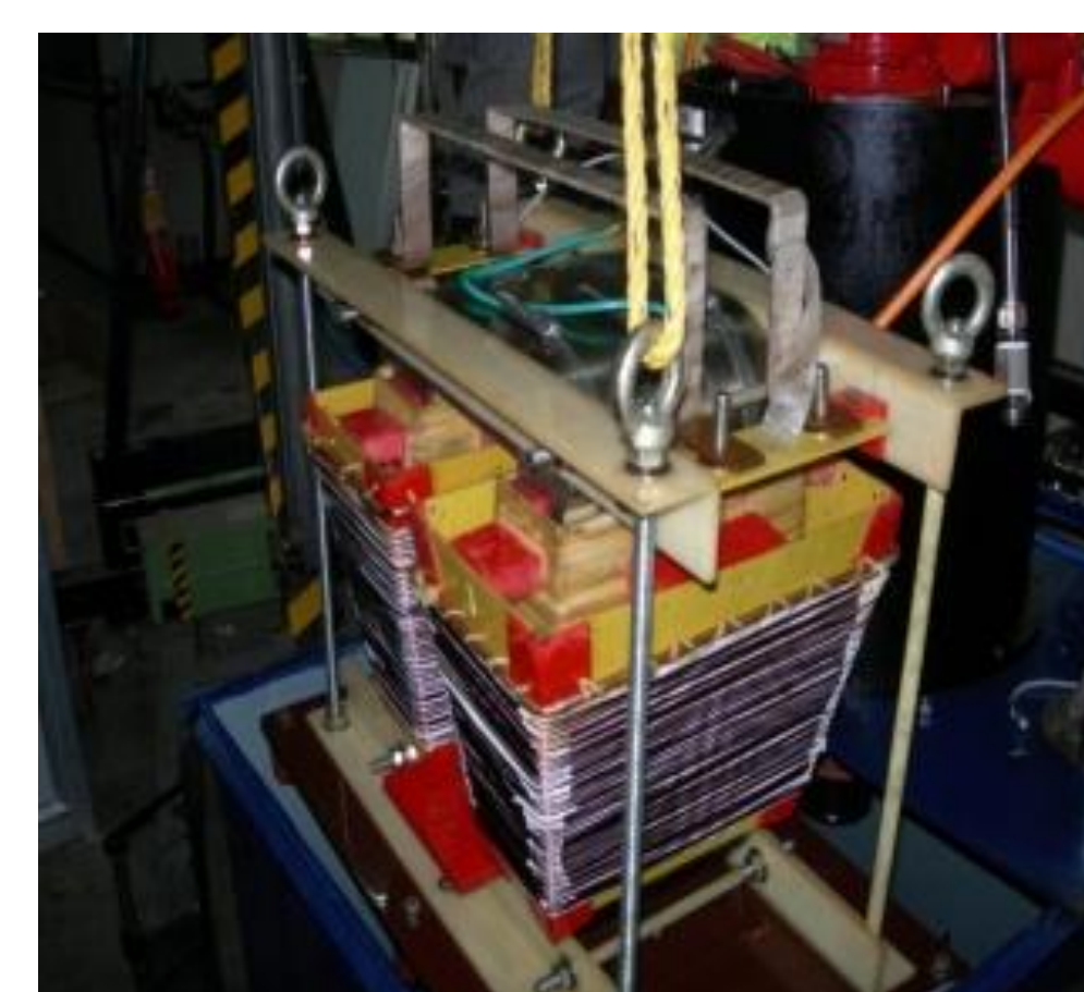
Pulse transformer (1:10.7) for 150kV/110 A klystron modulator
