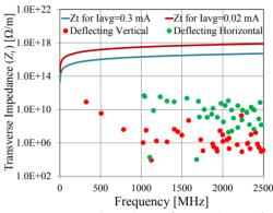
Figure 7: Transverse impedance from HOM and due to average beam current.
