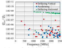
Figure 5:  $Q_{ext}$  as a function of mode frequency for the superconducting rf-dipole cavity.
