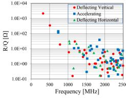
Figure 2: Mode spectrum of the superconducting rf-dipole cavity.
