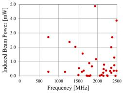
Figure 6: Induced beam power due to excitation of accelerating modes.
