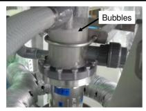
Figure 3: Picture of bubbles at upper side during VEP.
