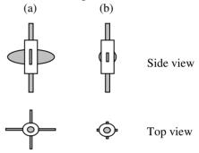
Figure 1: Schematic view of "i-cathode Ninia"®. (a) unfolded status. (b) retracted/folded status.
