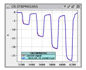
Figure 1: Beam current vs. time (ns), showing the fourfold increase during beam combination in the combiner ring. The two overlapping traces (red and blue) were taken on two different days, with identical machine settings.
