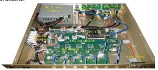
Figure 4: Field control chassis
