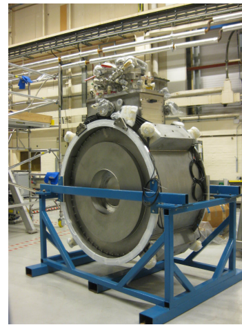
Figure 4: One of the MICE absorber focus coil modules at RAL.
