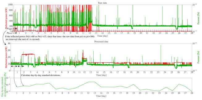
Figure 7: Reflected power and vacuum pressure of M04 in Feb. 2014. (Upper) Raw data. (Middle) After removing pressure fluctuations by an RF trip. (Bottom) Day-by-day standard deviations of the vacuum pressure.
