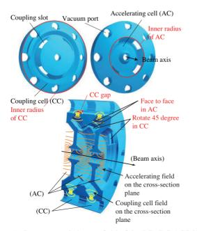
Figure 1: Structure and electric field of the J-PARC ACS [2].
