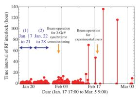
Figure 6: Long-term operation stability of M04.
