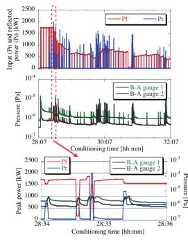
Figure 4: Detailed conditioning history around the time of the input power degradation due to an RF interlock.
