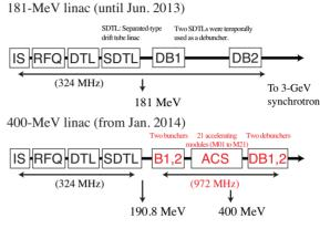
Figure 2: Configuration of the J-PARC linac.
