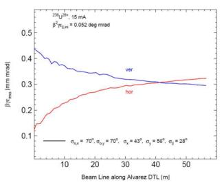
Figure 4: Normalized horizontal and vertical rms-emittances along the beam line. The assumed DTL is the artificially prolonged existing first tank A1, i.e. without inter-tank sections.
