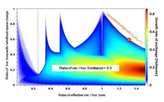
Figure 2: Stability chart for the ver/hor emittance ratio of 3.5 at the entrance to the existing Alvarez type DTL of the GSI UNILAC.
