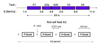
Figure 1: Scheme of the DTL (top) and its first cell (bottom).
