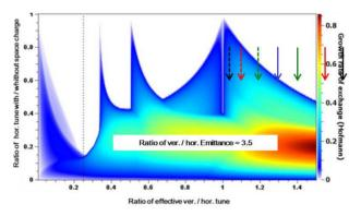
Figure 5: Stability chart and working points for the ver/hor emittance ratio of 3.5 at the entrance to the existing Alvarez type DTL of the GSI UNILAC assuming different focusing strength in the transverse planes.
