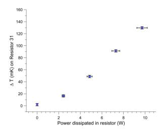
Figure 5: A plot of the temperature difference between the bath and the resistor located above the heater on the steel plate,  $\Delta T$ , as a function of the power dissipated in the heater. As expected, the dependence between power dissipated and  $\Delta T$  is linear.
