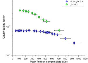
Figure 3: A plot of the quality factor of the cavity against the peak field on the surface of the sample plate, for two different ranges of the coupling  $\beta$ . The lower quality factor observed at higher coupling is due to losses in the coupler.
