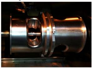
Figure 4: Cavity main body middle seam welding.
