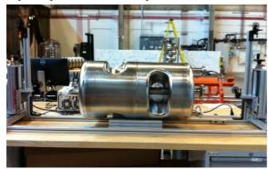
Figure 5: Complete cavity for bead pull set up.
