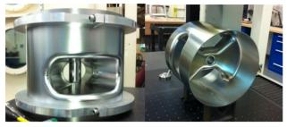
Figure 3: Weld fit-up and completed spoke-outer conductor subassembly
