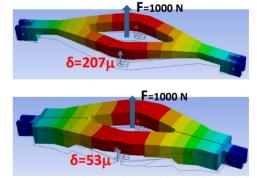
Figure 12: The original and the stiffened forks deflection due to bending.
