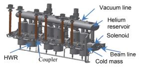
Figure 1: The inner parts of the 2.5 m long PSM.
