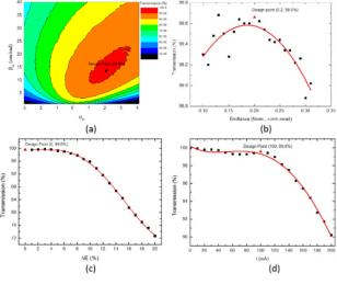
Figure 4: Transmission versus input twiss parameters (a), input beam emittance (b), input beam energy spread (c) and input beam current (d).
