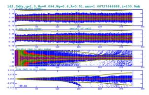
Figure 3: Beam dynamics in the RFQ for the input current of 100 mA, 10000 particles. From top to bottom are: x, y, phase, and energy coordinates versus cell number. The percentage transmission is 99.6%.
