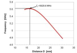
Figure 4: Cut-off frequency varying the distance D between two opposite ridges.
