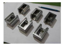
Figure 1: Sections of the cavity test used to determine the best magnetic steel for the load.
