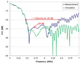
Figure 8: S11 frequency spectrum from cold measurement (blue line) e from analytical computation (green line).
