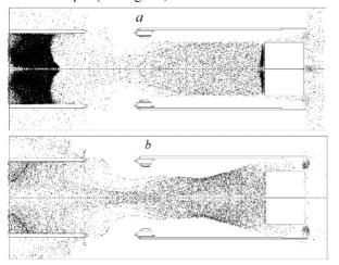
Figure 9: Electrons distributions for current 150mA (a) and  $150\mu$ A (b).
