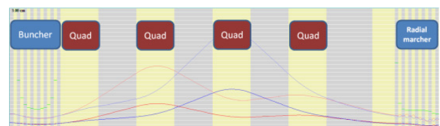
Figure 2: LEBT layout and simulated envelopes
