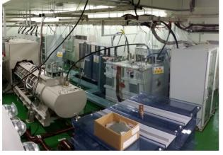
Figure 5: Photo of the 1.2 MW, 324 MHz klystron and its modulator power supply.
