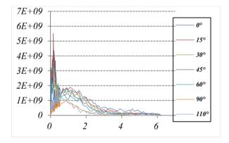
Figure 3:  ${}^{9}Be(p,n){}^{9}B$  Neutron energy spectrum (n/cm<sup>2</sup>/mA/sec) as a function of  $E_n$  (MeV) for a 8 MeV primary proton beam on a 3 mm thick beryllium target for various production angles.
