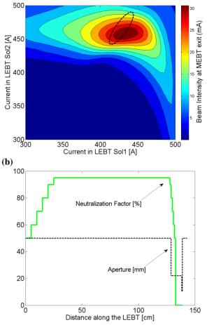
Figure 6: (a) Simulated beam intensity at the MEBT exit as a function of the LEBT solenoid currents for (b) a nonuniform neutralization along the LEBT. From TRACK. The ellipse mimics the measured area of favorable transmission reported in Fig. 2.
