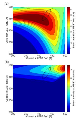
Figure 3: Simulated beam intensity at the MEBT exit as a function of the LEBT solenoid currents for a uniform neutralization factor along the LEBT of (a) 100% and (b) 60%. From TRACK. The ellipse mimics the measured area of favorable transmission reported in Fig. 2.
