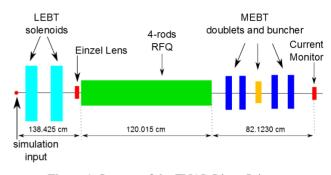
Figure 1: Layout of the FNAL Linac Injector.
