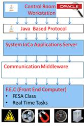
Figure 2: Three tier architecture
