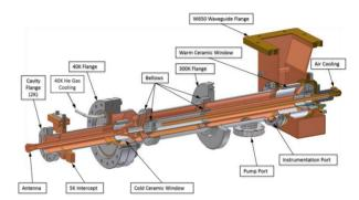
Figure 5: Main linac coupler design.
