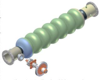
Figure 4: A 7-cell cavity with input coupler.
