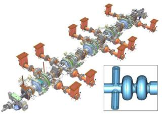
Figure 1: Injector cavities with input couplers.
