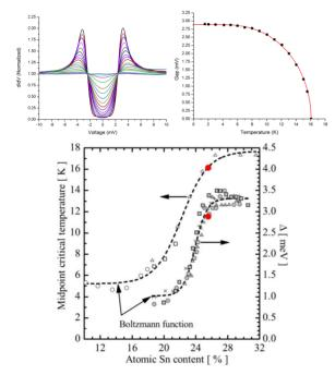
Figure 5: Top left: Point contact tunneling measurements made at several different temperatures. Top right: extraction of  $T_c$  and  $\Delta$ . Bottom: Comparison of extracted values (red) to literature with figure adapted from [5].
