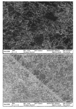
Figure 2: Large grain niobium coated with Nb<sub>3</sub>Sn appears to have some regions with large "clumps" along with the usual grains. Shown is a sample coated without nucleation agent, both far from (top) and including (bottom) a grain boundary of the LG substrate. The niobium grain boundary's influence on the grain structure of the Nb<sub>3</sub>Sn is clearly observed.
