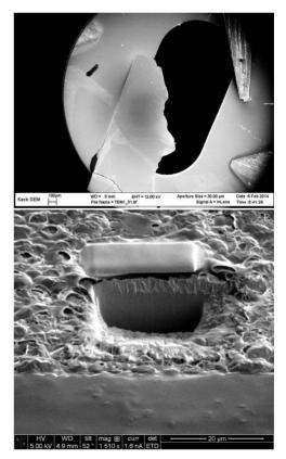
Figure 4: Attempts to make TEM-transparent samples via mechanical polishing with a diamond lapping film (top) and ion milling (bottom). Further effort will be needed to extract usable TEM samples.
