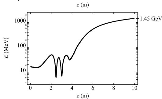
Figure 2: Energy of the electron beam gained along a 10 m long plasma cell [15].
