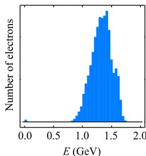
Figure 3: Energy distribution of the accelerated electron beam after 10 m plasma.
