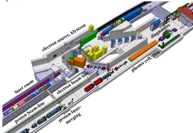
Figure 5: Integration of the AWAKE experiment in the experimental area at CERN.
