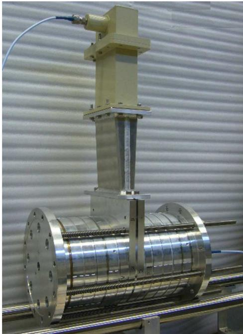
Figure 4: Half size model of ACS with direct RF feed.
