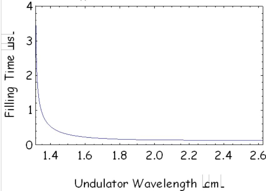
TE<sub>12</sub> Mode at 11.424 GHz for K=1
