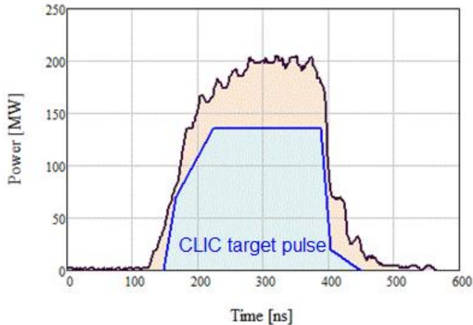
After start up and initial conditioning, PETS was reliably generating RF peak power well in excess of the CLIC nominal value.
