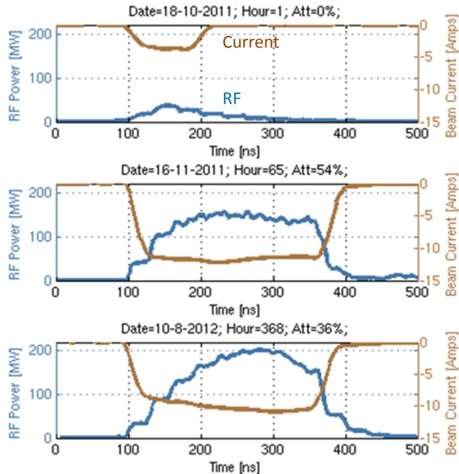
Typical drive beam current and RF power pulses at the different stages of operation.
