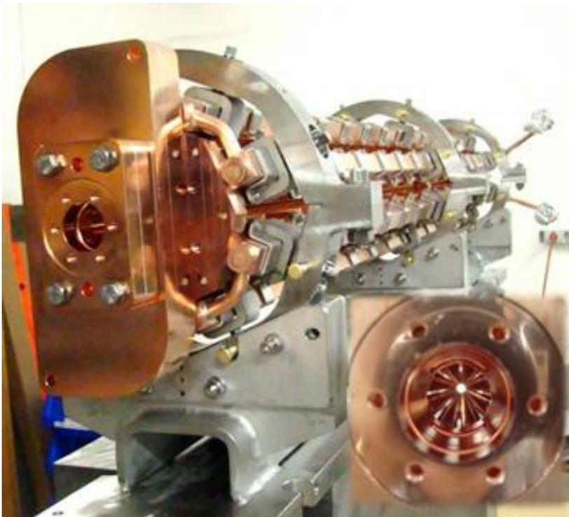
The fully assembled, 1 meter TBTS PETS equipped with water cooling channels and power couplers on its girder and ready for the installation into the vacuum tank.
