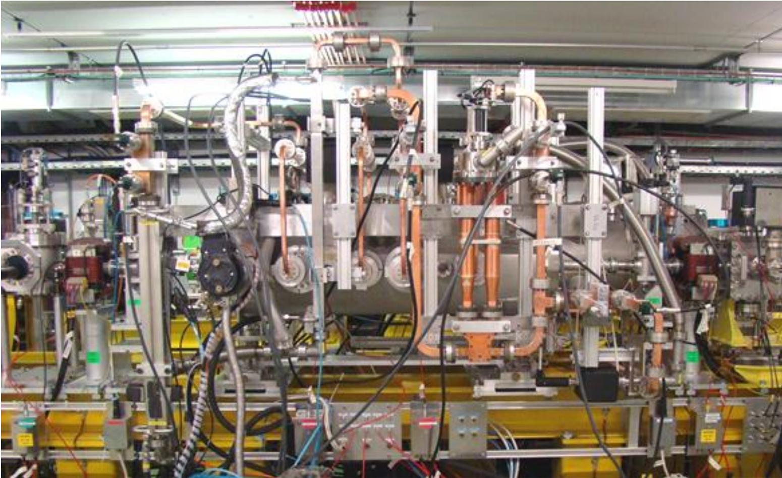
The new tank with two accelerating structures is installed and connected to the PETS
