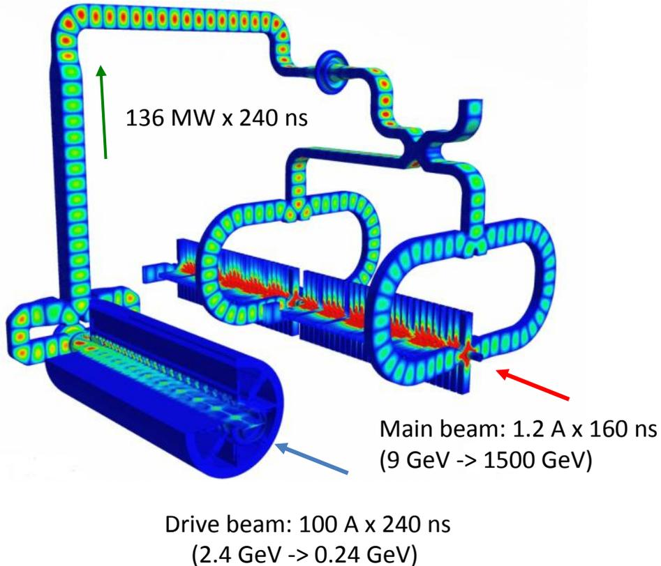
The two beam acceleration is one of the key component of the CLIC scheme, where the RF power is produced via deceleration of the high current, low energy drive beam and then is used to accelerate the low current main beam to high energy.
