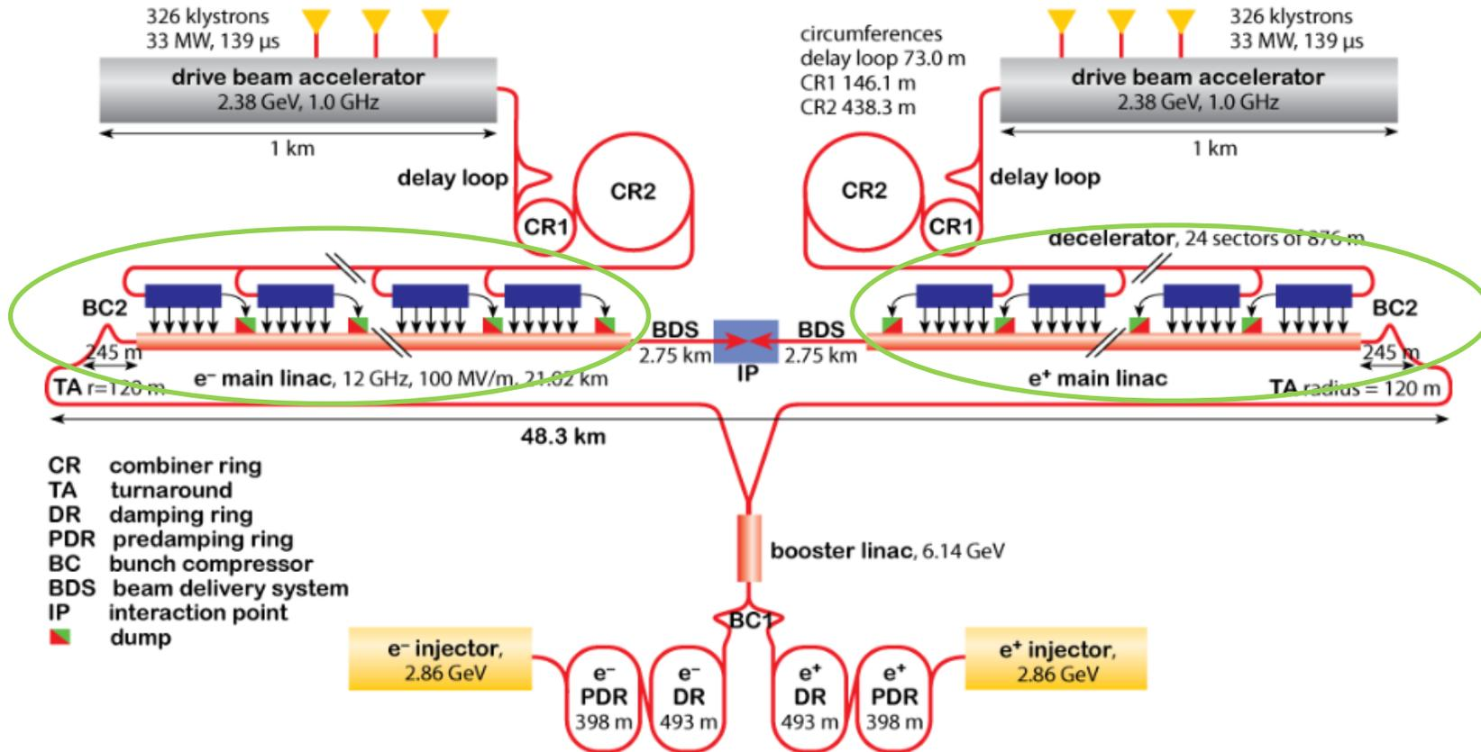
In the CLIC linac, 24 decelerator sectors (each 876 m long) should produce 2.8 TW peak RF power in total, in order to accelerate the main beam to from 9 GeV to 1.5 TeV. Notably, the efficiency of the RF power production is 90%.
