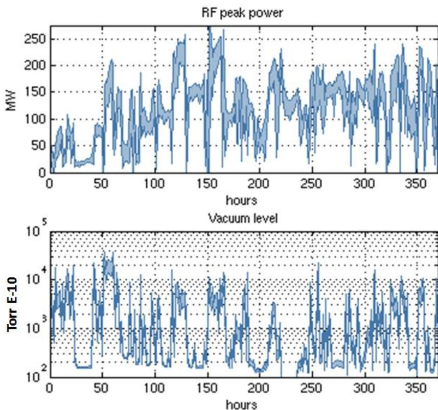
To demonstrate the power capability of the new RF components used in the ON/OFF RF circuit, we set the recirculation loop parameters to their amplification mode.
