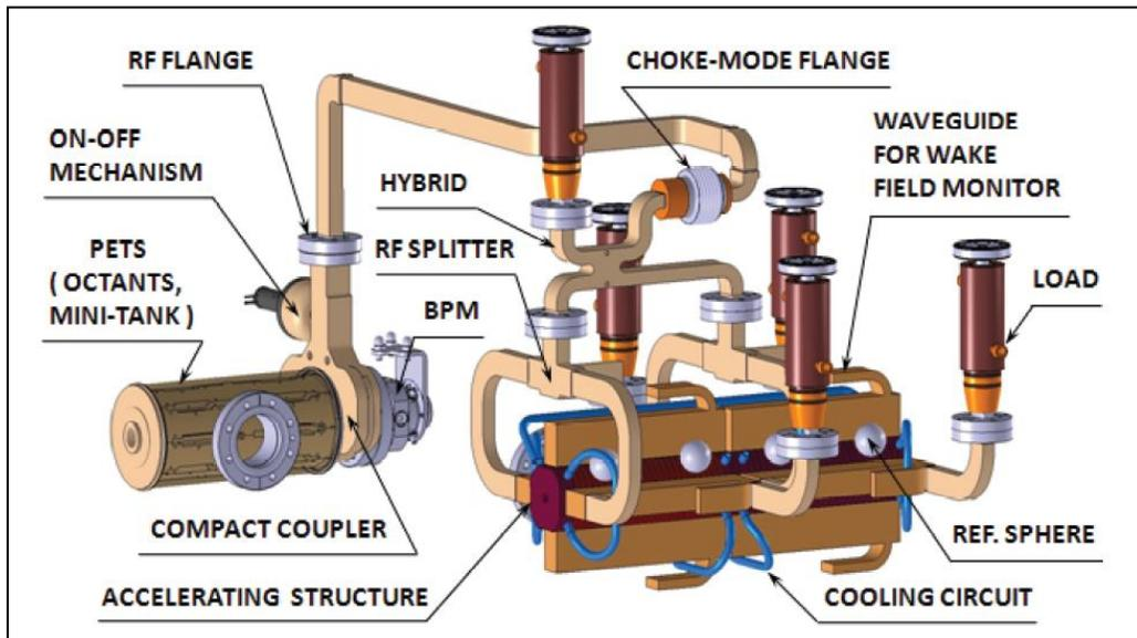
Depending on its type, each module contains up to 4 RF units. Each RF unit comprises of Power Extraction and Transfer Structure (PETS) and two accelerating structures connected via special RF waveguide network.
