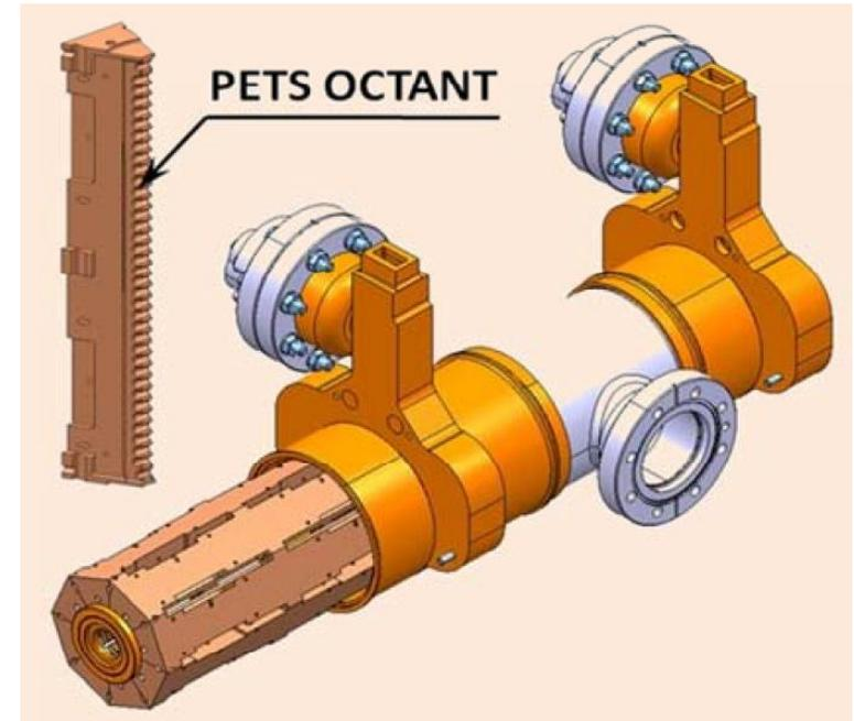
Depending on its type, each module contains up to 4 RF units. Each RF unit comprises of Power Extraction and Transfer Structure (PETS) and two accelerating structures connected via special RF waveguide network.
