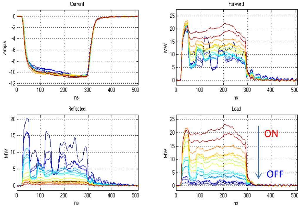
During experiments with the beam, the variable reflector settings were changed gradually from full reflection to full transmission. The results were in a good agreement with the system computer modeling, where measured S-parameters of all components were used as an input.
