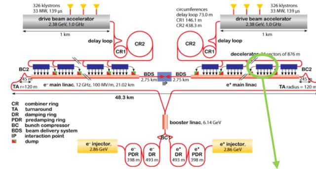
Each decelerator sector is comprised of 438 Two-Beam Modules (TBM). The TBM is a complicated installation, where all the accelerator systems and components are integrated in a very compact way.
