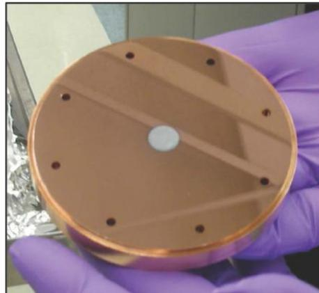
**2  $\mu$ m of Mg is sputtered in a 1 cm diameter spot on the Cu back plane of the photoinjector**
