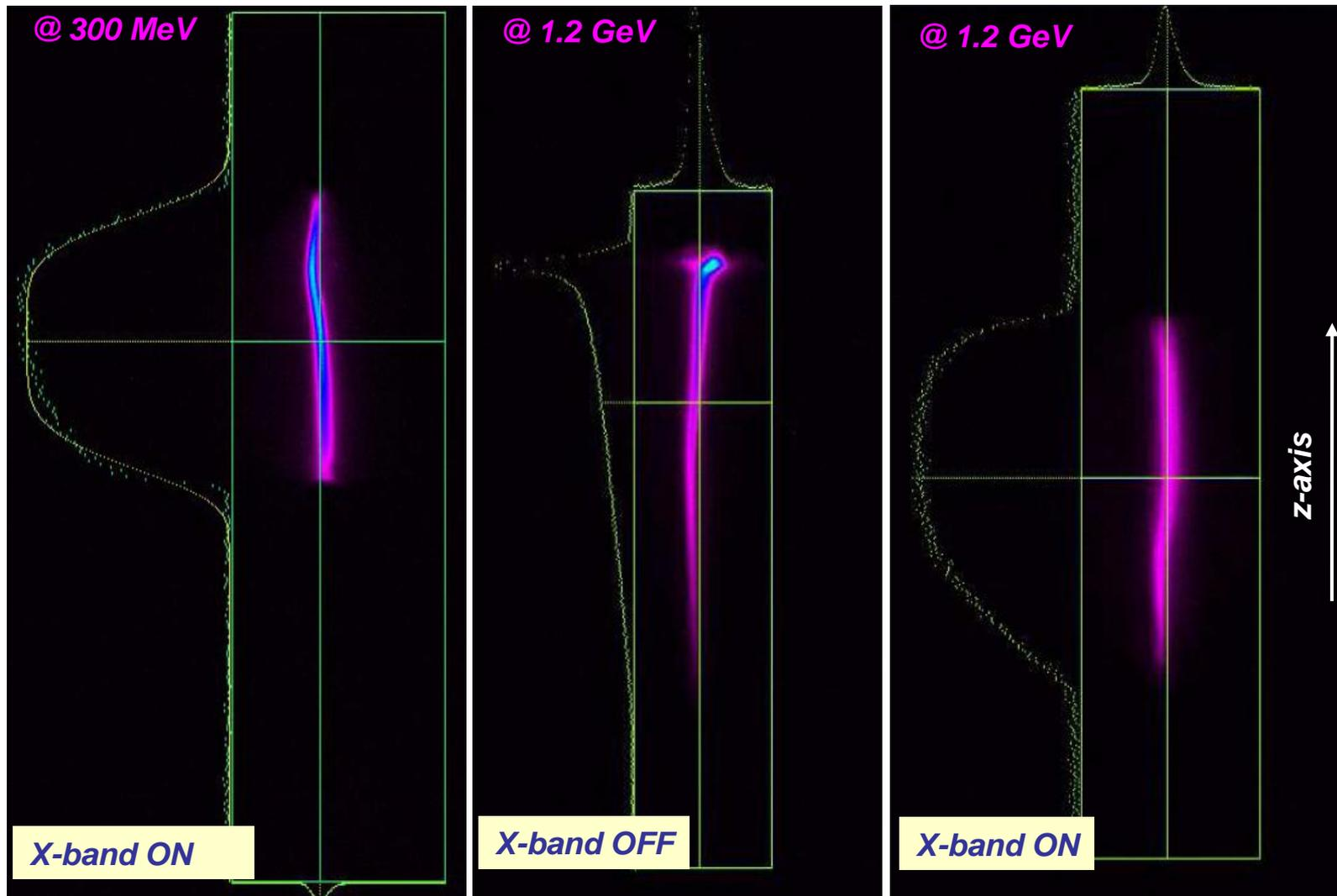
Slice beam analysis made @1.2 GeV using a high energy TDC
