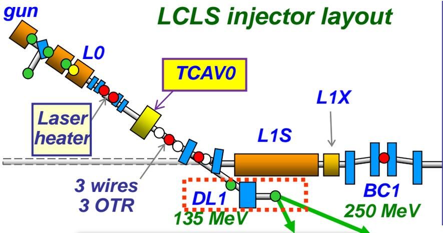
The diagnostics is further enhanced if the deflected beam is observed on an energy spectrometer screen, where the energy dispersion is in the plane perpendicular to the RF deflection. The dispersion properties of the dipole allow for the complete characterization of the energy distribution of each bunch slice reconstructing the longitudinal phase space.
