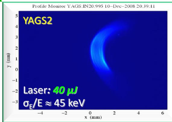
Energy profile and slice energy spread measurements with TCAV at LCLS
