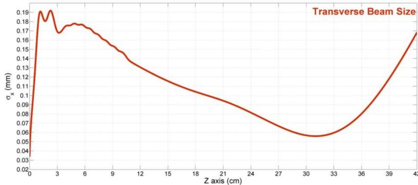
**Beam Size Controlled with Solenoids**
