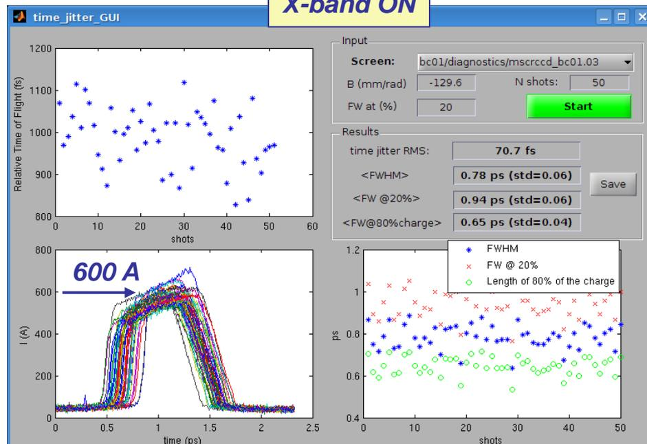
**Bunch temporal profiles with and without X-band downstream BC1, using a TDC@300 MeV. Analysis on 50 shots**
