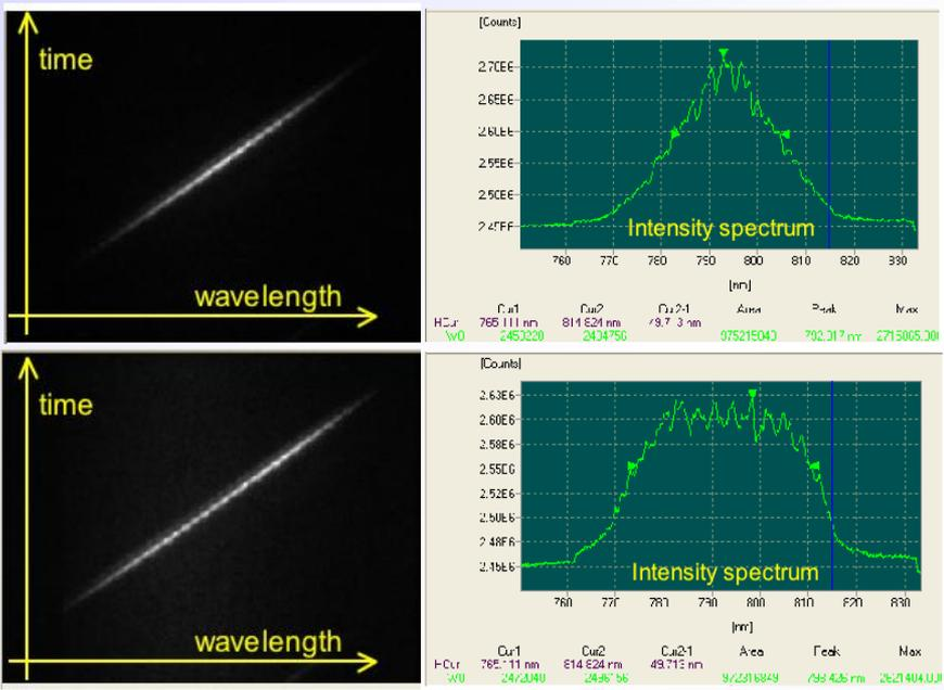
Measurements of linear-chirped laser probe pulse with Spectrograph Streak camera:
