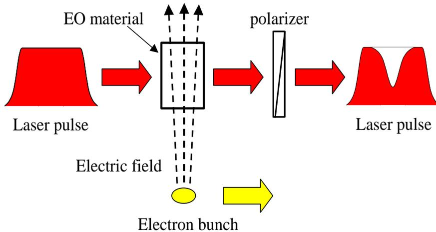
Refractive index inside EO crystal changes when Coulomb field is applied.
