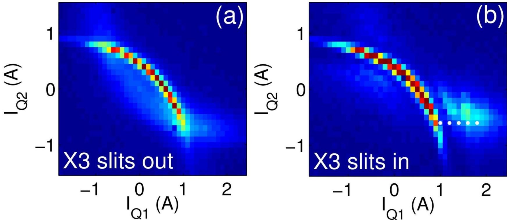
The final beam longitudinal properties can be controlled by initial horizontal beam parameters.
