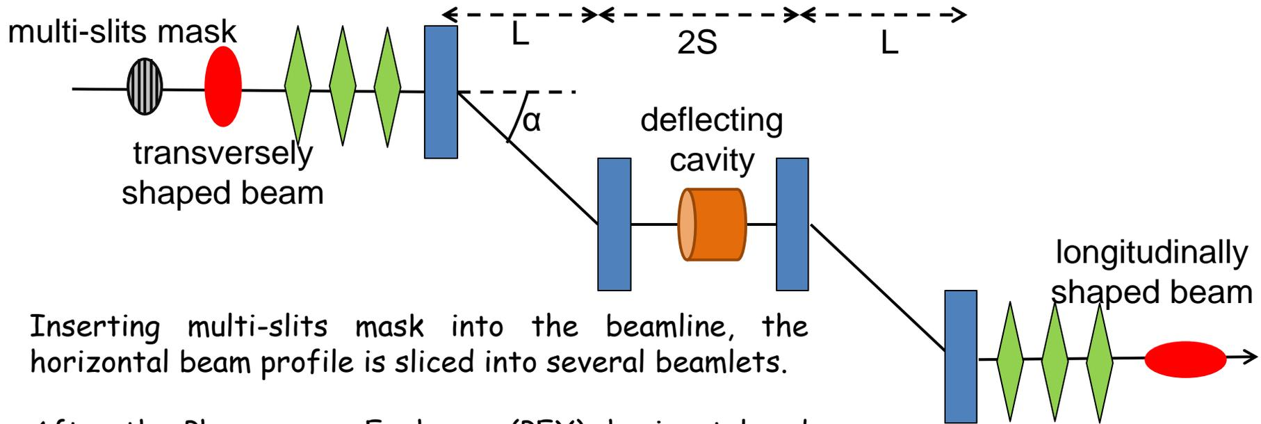
Inserting multi-slits mask into the beamline, the horizontal beam profile is sliced into several beamlets.
