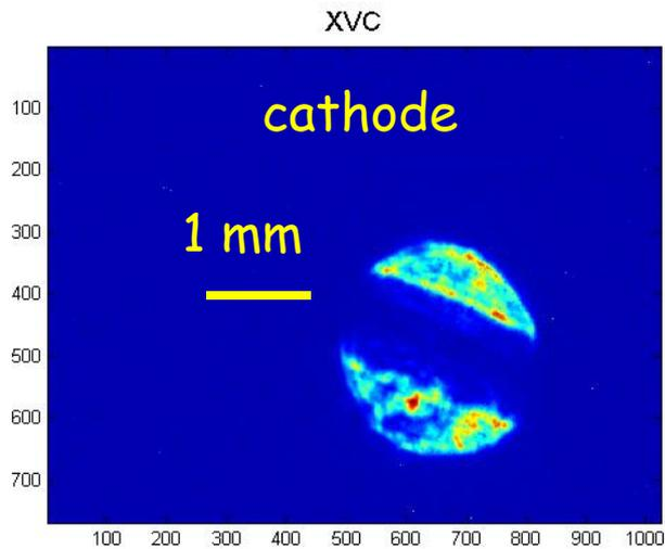
By inserting a 1mm diameter rod into the photo-cathode drive laser, the beam is divided into two beamlets on the cathode, then transported through the EEX beamline.
