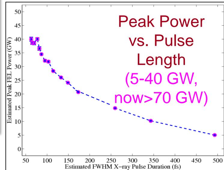
$e^-$  bunch length is quickly adjustable (<1 min) from 60 to 500 fs (hard x-rays: 60 to 100 fs)
