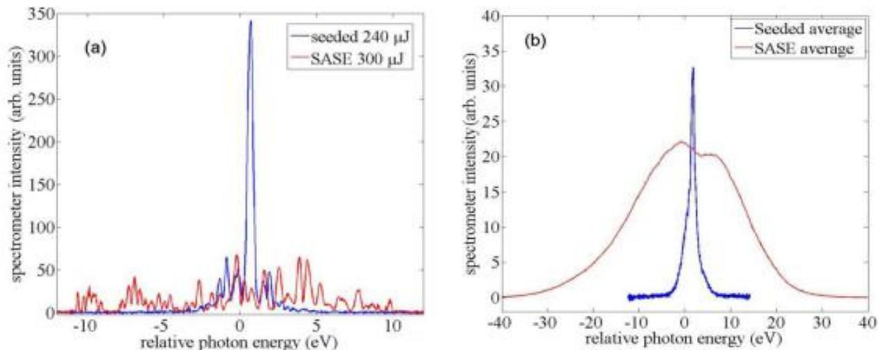
**Figure 5.** Single-shot (a) and averaged (b) x-ray spectrum in SASE mode (red) and self-seeded mode (blue). The FWHM single-shot seeded bandwidth is 0.4 eV, whereas the SASE FWHM bandwidth is approximately 20 eV. Vertical scales have the same arbitrary units in both plots (a) and (b). The chicane is turned off for the SASE measurements, but necessarily switched on for the self-seeded mode.
