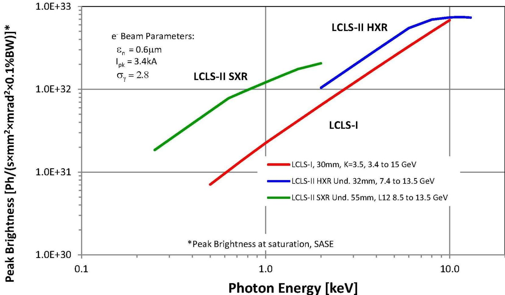
Tuning the X-Rays with both undulator gap and Electron Beam Energy
