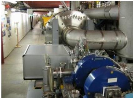
> Normal conducting 1.3 GHz RF gun
