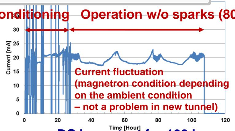
DC beam test for 100 hrs
