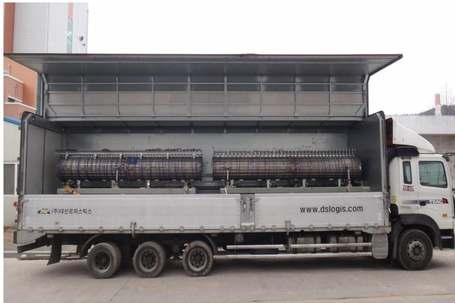
DTL tanks inside vibration free truck
