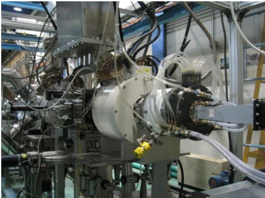
Microwave ion source installed in 20-MeV linac
