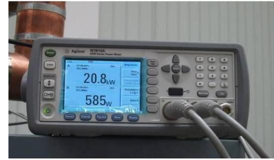
**Coupler power exceeds 20 kW (CW, designed value), 2012.7**
