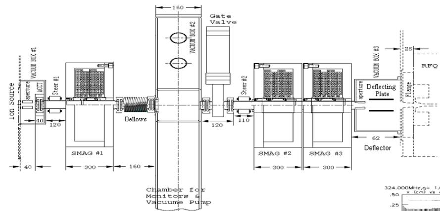
A Penning H- ion source and a three-solenoids LEBT with space charge neutralization.
