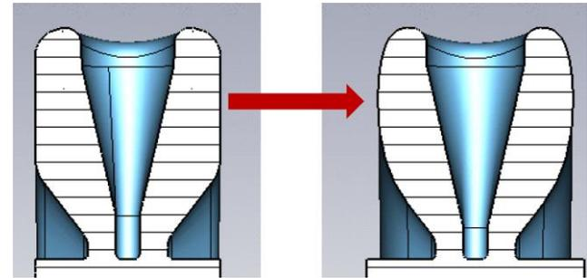
The Convex end wall (right) is adopted, which has better mechanical performance than the flat one (left).
