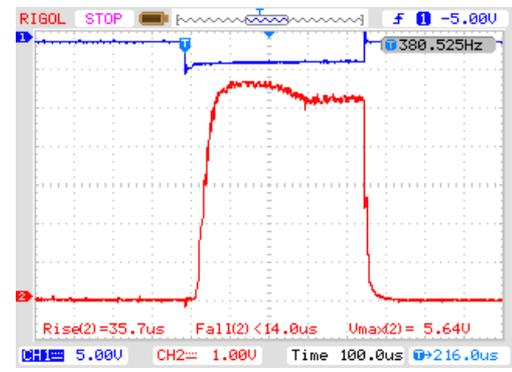
Phase space and proton pulse measured at the end of the LEBT.
