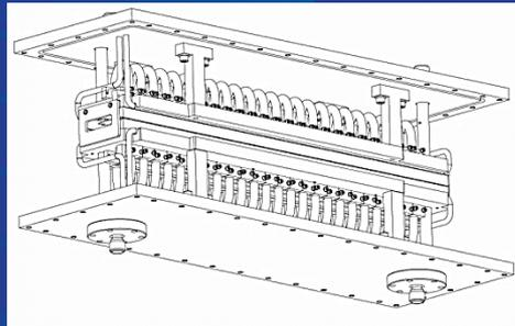
Mechanical schematic of a 50-Ohm kicker
