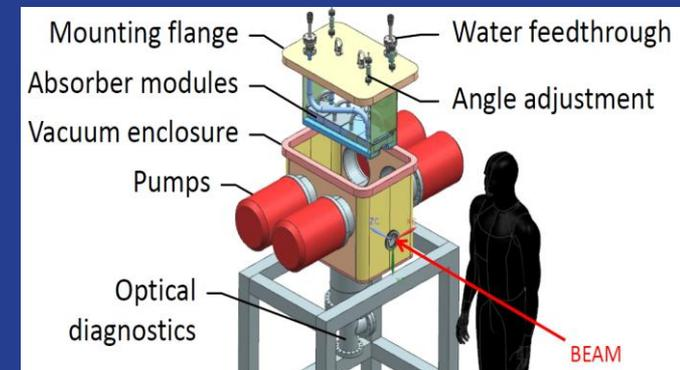
MEBT absorber: TMZ alloy, 40 cm long. Requirements: 21 kW beam,  $\sim 2$ mm rms rad, 29 mrad grazing angle.
