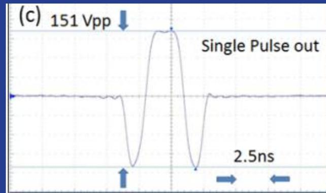
Test of a 150-W amplifier as a kicker driver: output signal for a single pulse
