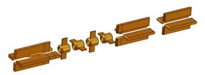
The main feature of the RFQ is the new approach to the beam formation at the RFQ output that provides converging beam in both transverse planes as well as in longitudinal one. It is achieved by adding after regular RFQ vanes several drift tubes and RF quadrupoles that act as triplet. RFQ output beam can be directly injected into DTL cavity.
