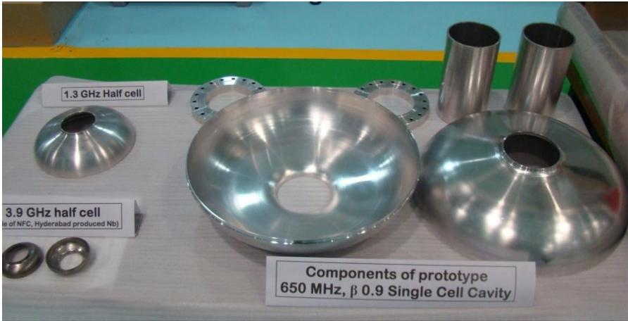
Prototype 3.9 GHz, 1.3 GHz and 650 MHz cavity development
