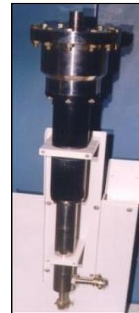
30 kW RF Dummy Load
