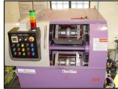
Centrifugal barrel polishing machine
