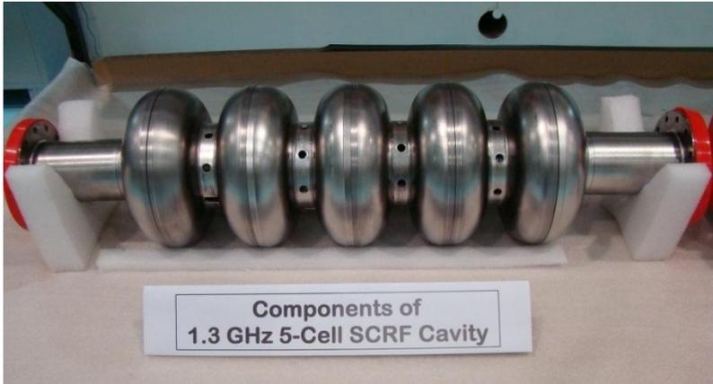
Prototype 1.3 GHz, 5-cell SRF Nb cavity
