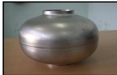
Prototype 1.3GHz cavity
