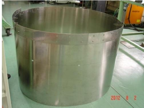
External Magnetic Shield segment under fabrication
