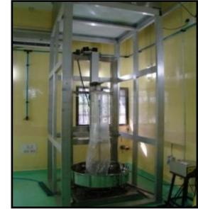
High pressure rinsing Set up
