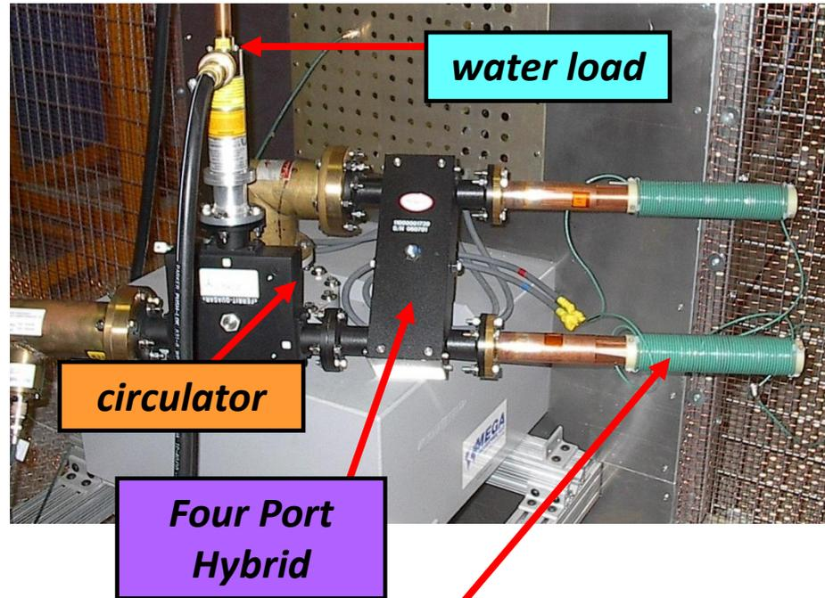
*Modulates phase and amplitude independently:*
