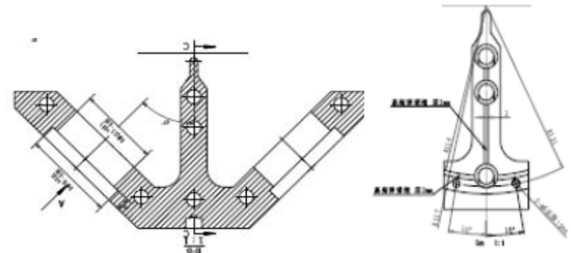
324MHz RFQ cavity is resonantly coupled by two segments and each segment is divided into two modules (left). Each module is composed of two major vanes and two minor vanes with cooling-water channels (right).
