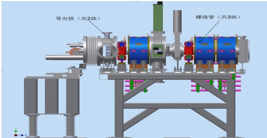
A Penning H- ion source and a three-solenoids LEBS with space charge neutralization. Pre-chopper is mounted at the entrance of the RFQ with a beam rise time of 15ns.
