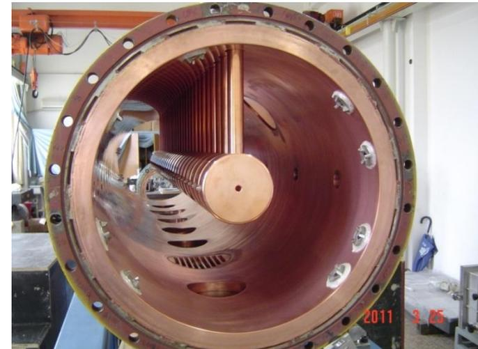
A prototype DTL has been fabricated for the technology development and cold measurement.
