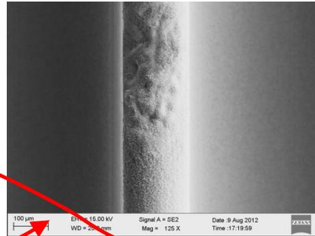
1<sup>st</sup> iris – **breakdown damage**, peak surface fields < 1.3 GV/m
