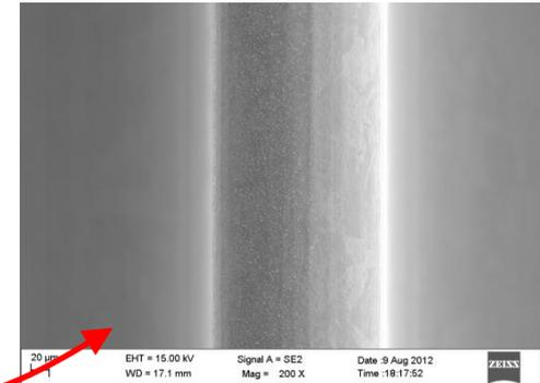
9<sup>th</sup> iris – **no breakdown damage**, peak surface fields > 0.64 GV/m, pulse length ~3ns
