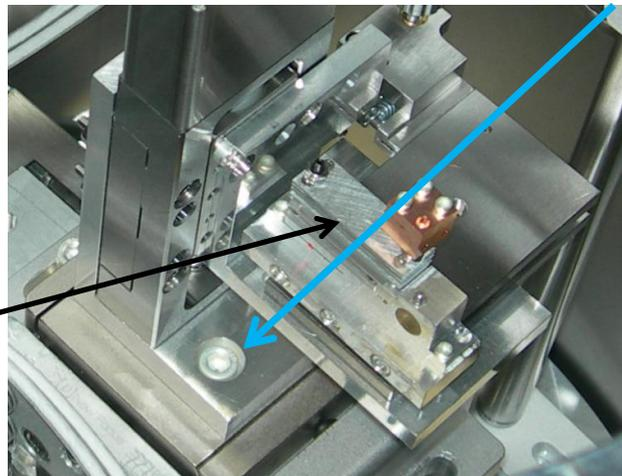
e- The FACET beam is sent through prototype structures of varying dimensions and materials
