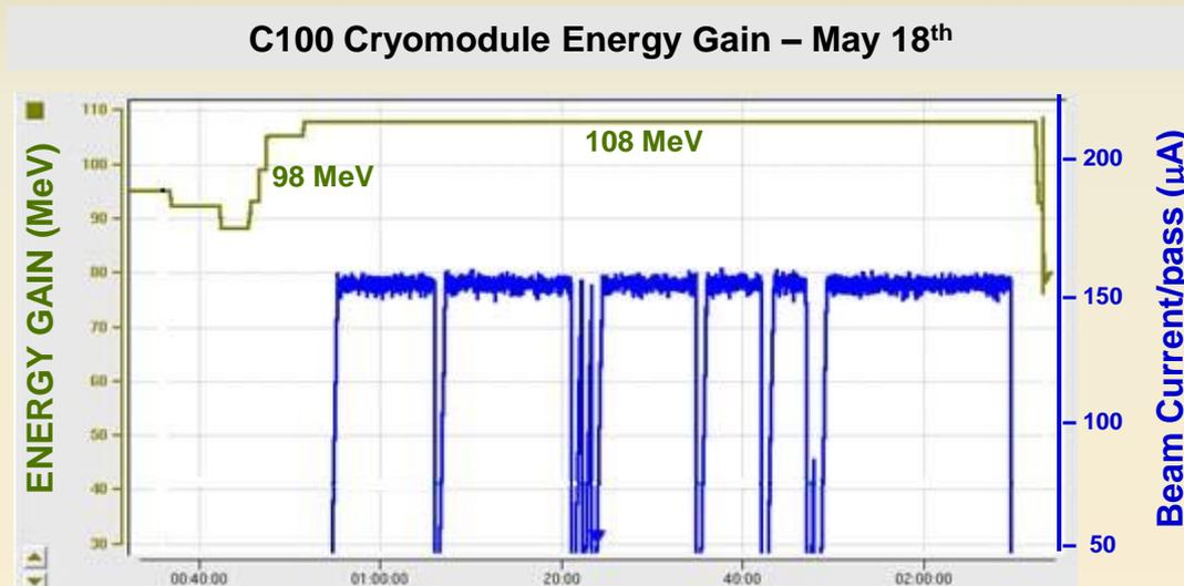
C100 reached design energy gain (108 MeV) for the nominal 12 GeV current of 465  $\mu\text{A}$  on May 17 2012.
