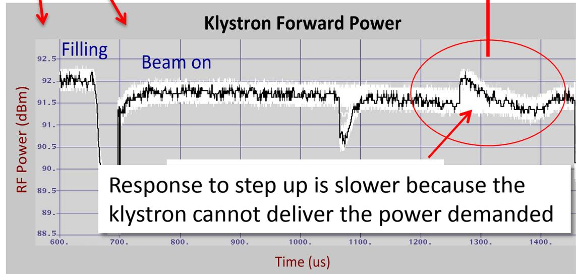
Response to step up is slower because the klystron cannot deliver the power demanded
