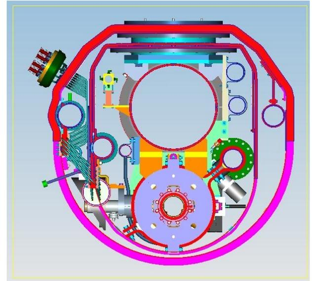
Conduction cooling through Al-strips
