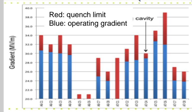
The limiting cavity is within 5% of quench
