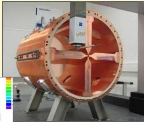
T5 segment - 3D measurements
