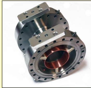
Part of TOF device (exit of the linac)
