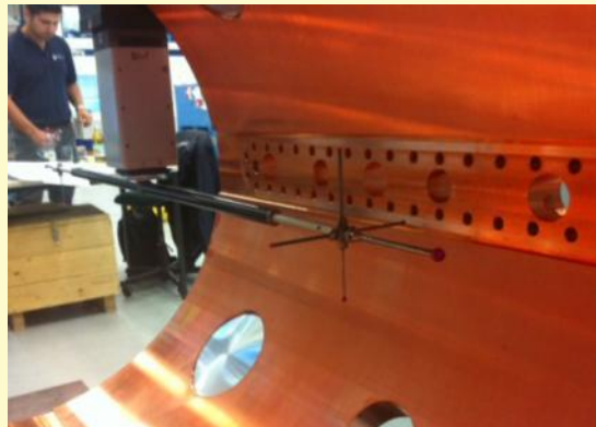
3D Measurement of tubes T1..T4
