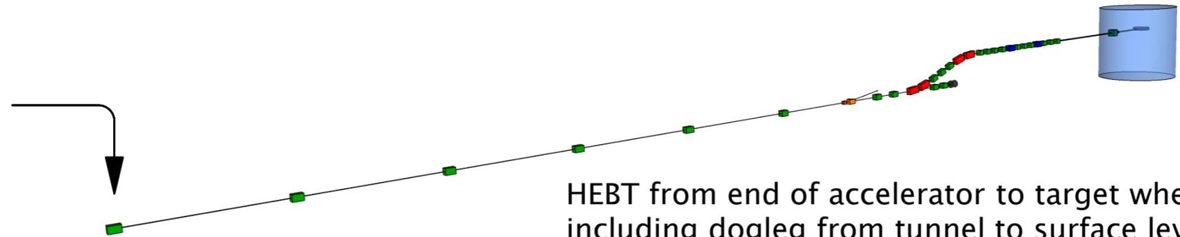
HEBT from end of accelerator to target wheel, including dogleg from tunnel to surface level, expansion magnets and tuning beam dump.
