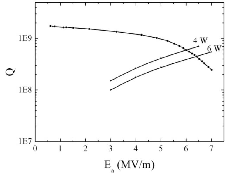
Resonator Q as a function of the accelerating gradient  $E_a$  at 4.2 K
