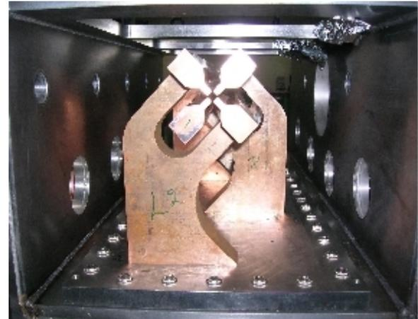
**RFQ Prototype with Cu plated ss tank, Cu vanes tested upto 26 kW**
